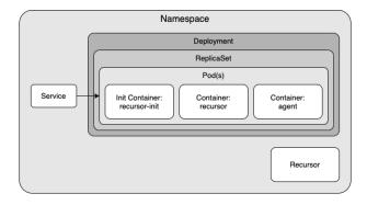
As the diagram shows a Recursor pod will consist of 2 containers + 1 init container:
