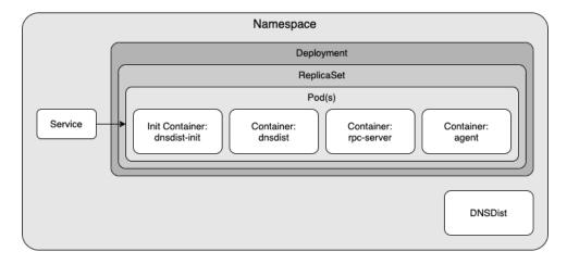
As the diagram shows a DNSdist pod will consist of 3 containers + 1 init container:
