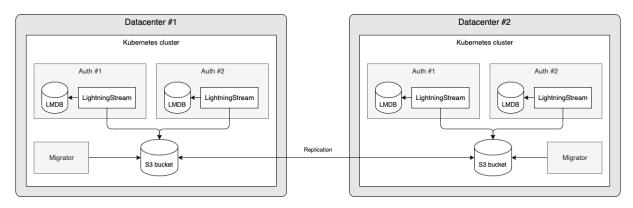
Because of the Migrator pod, you can safely upgrade Cloud Control in each datacenter sequentially. When you upgrade datacenter #1, all known data will be migrated to a new schema version (if required) and any writes handled by the deployment in datacenter #2 (old schema version) will be migrated, albeit with a minor delay of 10-15 seconds. Once all deployments are upgraded to the same version, the Migrator will no longer have anyhing to do and will idle until a new upgrade is detected.
