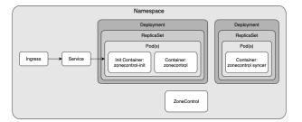
As the diagram shows a ZoneControl instance will consist of a ZoneControl deployment with 1 container + 1 init container and a ZoneControl Syncer deployment. The ZoneControl Deployment contains the GUI and can have multiple replicas, while the ZoneControl Syncer deployment has a single replica and is used to synchronise configuration changes to the ZoneControl instances.
