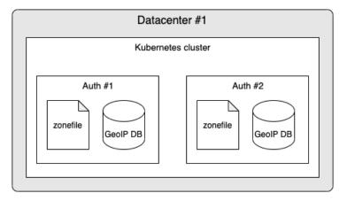
Since the Auth instances have a copy of the zonefile(s) and GeoIP databases locally, you can replicate this deployment across multiple datacenters simply by deploying the same configuration to each datacenter.
