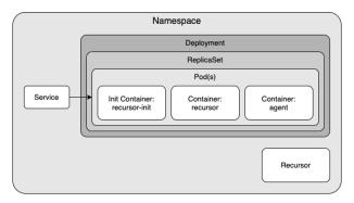
As the diagram shows a Recursor pod will consist of 2 containers + 1 init container:
