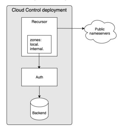
In this setup we tell Recursor to forward all traffic for zones matching 'local.' and 'internal.' to a set of Auth instances, while the rest of the traffic will be handled as per default resolution via public nameservers. To configure this scenario, you can use the following forwarding configuration:
