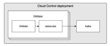
When deployed as a sidecar in a Recursor pod with a Kafka destination:
