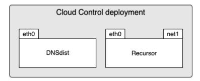
By default, the Recursor will not make efficient use of the additional interface though, as Kubernetes default routing will prioritise the pod network's eth0. To force the Recursor to use the additional interface for outbound traffic you can configure the 'outboundInterfaces' parameter, for example:
