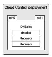
The defaults for this scenario are slightly different, since Recursor is embedded within the Dnsdist pod. The enabled traffic flows are:
